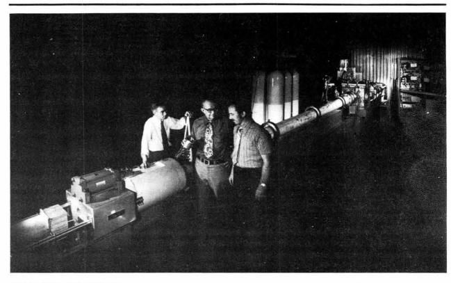
RECOVERED PROJECTILE from previous gas gun experiment is examined by (from left) Wil Vandermolen, Dick Jacobson and Ralph Thompson (all 8414). Data acquisition system is at far right.
